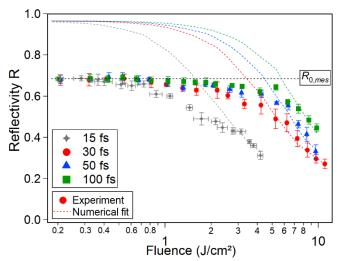
Figure 6. Evolution of the reflectivity calculated with the Drude model, compared to the experimental results for the four pulse durations.
