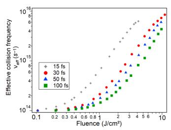
Figure 8. Evolution of the effective collision frequency  $\nu_{eff}$  as a function of the incident fluence and for the four pulse durations studied.
