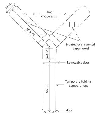
Fig. 1. Diagram of the Y-maze used for experiments.
