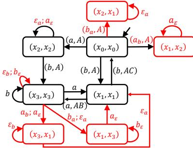
Fig. 5. Composed automaton  $G(f) = G_C(f) \times G_A(f)$ .
