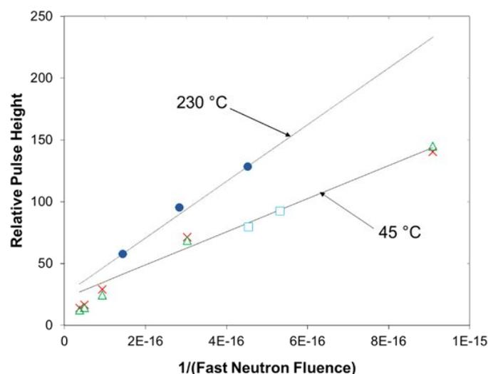
Fig. 14. Effect of elevated temperature during neutron irradiation on the observed pulse heights from a <sup>238</sup>Pu alpha test source. Pulse height is plotted as a function of reciprocal fast neutron fluence. The symbols refer to different irradiated SiC detectors. (Figure adapted from Reference 55)
