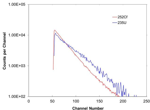
Fig. 6. Comparison of the response spectra of a SiC detector to neutron-induced fission neutrons from  $^{235}\text{U}$  and  $^{252}\text{Cf}$  spontaneous fission neutrons. (Adapted from Reference 36)
