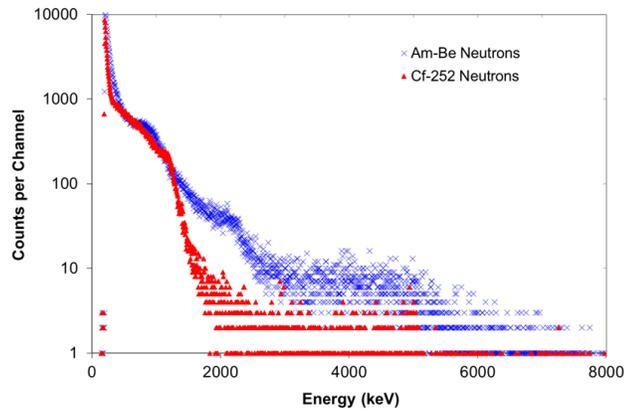
Fig. 5. Comparison of the responses of a SiC detector to fission neutrons from  $^{252}\text{Cf}$  and neutrons from an  $^{241}\text{Am}$ -beryllium source. (Adapted from reference 25)
