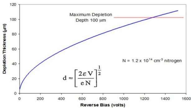
Fig. 3. Depletion depth as a function of applied reverse bias for a 100- $\mu\text{m}$  thick epitaxial layer with a nitrogen concentration of  $1.2 \times 10^{14} \text{ cm}^{-3}$ . The maximum depletion depth (horizontal red line) is the thickness of the epitaxial layer. A reverse bias of 1200 v is required for full depletion. If the reverse bias is limited to 1000 v, a 90- $\mu\text{m}$  depletion depth results.
