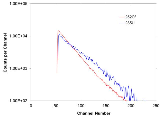
Fig. 6. Comparison of the response spectra of a SiC detector to neutron-induced fission neutrons from  $^{235}\text{U}$  and  $^{252}\text{Cf}$  spontaneous fission neutrons. (Adapted from Reference 36)
