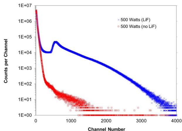
Fig. 4. Comparison of the neutron response of a 500- $\mu\text{m}$  diameter  $\times$  3- $\mu\text{m}$  SiC Schottky diode to reactor fission neutrons with and without a 24.2- $\mu\text{m}$   $^6\text{LiF}$  converter foil. With the  $^6\text{LiF}$  foil present, the detector response is primarily to thermal neutrons. When the  $^6\text{LiF}$  foil is absent, the detector responds primarily to fast neutrons. (Figure reproduced from Reference 32).
