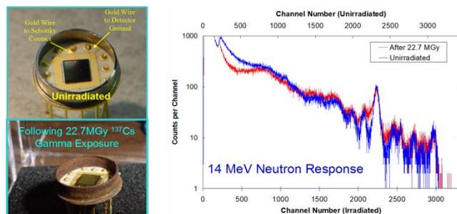
Fig. 10. Photographs of a 6-mm<sup>2</sup> x 100- $\mu\text{m}$  SiC Schottky diode before (top) and after (bottom) exposure to a cumulative  $^{137}\text{Cs}$  gamma-ray dose of 22.7 MGy and comparison of the corresponding neutron responses (Figures adapted from reference 48)
