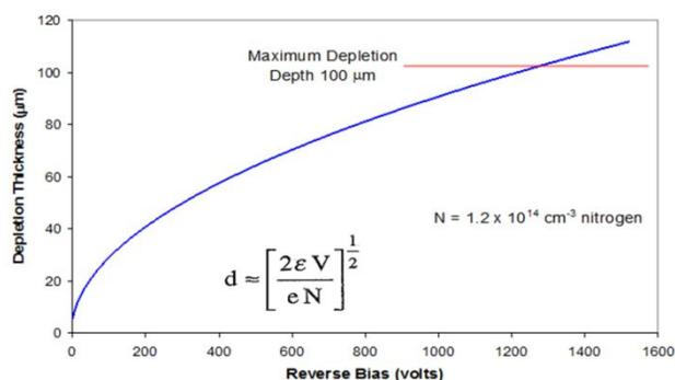
Fig. 3. Depletion depth as a function of applied reverse bias for a 100- $\mu\text{m}$  thick epitaxial layer with a nitrogen concentration of  $1.2 \times 10^{14} \text{ cm}^{-3}$ . The maximum depletion depth (horizontal red line) is the thickness of the epitaxial layer. A reverse bias of 1200 v is required for full depletion. If the reverse bias is limited to 1000 v, a 90- $\mu\text{m}$  depletion depth results.
