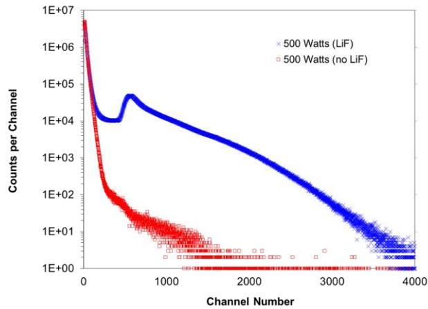
Fig. 4. Comparison of the neutron response of a 500- $\mu\text{m}$  diameter  $\times$  3- $\mu\text{m}$  SiC Schottky diode to reactor fission neutrons with and without a 24.2- $\mu\text{m}$   $^6\text{LiF}$  converter foil. With the  $^6\text{LiF}$  foil present, the detector response is primarily to thermal neutrons. When the  $^6\text{LiF}$  foil is absent, the detector responds primarily to fast neutrons. (Figure reproduced from Reference 32).
