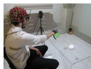
Figure 1: Participant with finger-tracking device manipulating virtual object.
